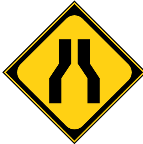
Width of Road Reduced
